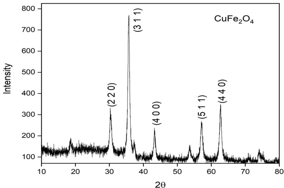
Fig. 1. XRD pattern  $\text{CuFe}_2\text{O}_4$  thin film
