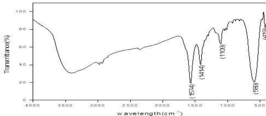
Fig. 2. FTIR pattern  $\text{CuFe}_2\text{O}_4$  nanoparticles
